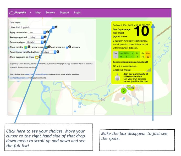
Raw PM2.5 Data. Use this filter often - it shows the smallest and most harmful particle size and it's not adjusted to fit some formula!
