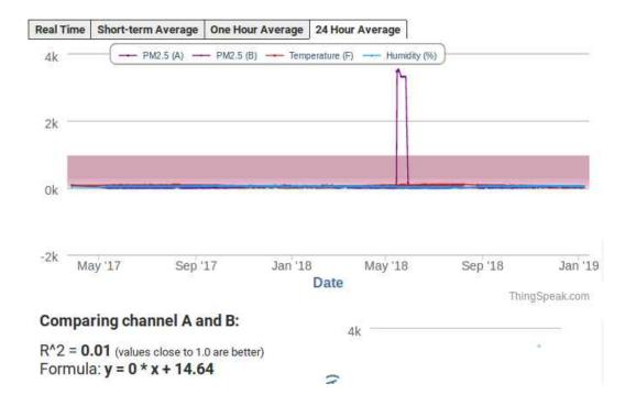
The vertical blip was apparently caused by a stuck fan on one channel. The unit was removed from service on May 13, 2018 and not returned until August. The presence of readings in the archive for the intervening period does not indicate Hazelton conditions, but those in my office where the unit was being tested. *Caveat emptor.* Spreadsheet values given below are for two ranges, Jan 1-May 10 then Sept 1-Dec 31.
