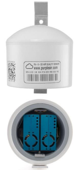
PurpleAir LCM - ~1300 in Canada (2x Plantower PMS5003)
